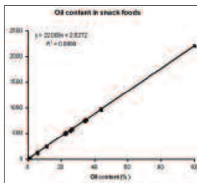
Figure 1: Correlation between NMR signal/mass and reference values
